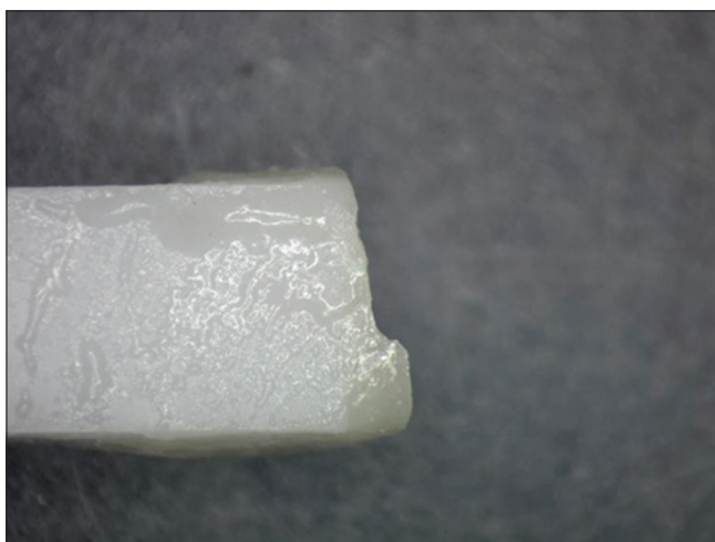
Figure 8: Combined failure mode
