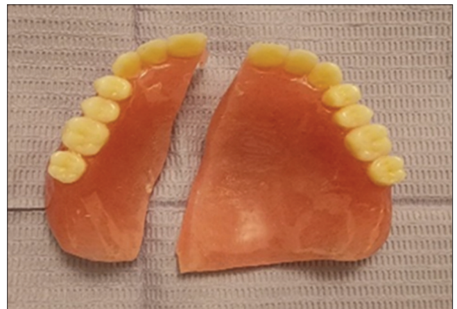
Figure 7: Unreinforced maxillary denture fracture
