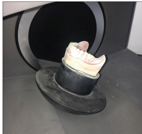
Figure 4: Scanning of the lower denture on desktop scanner
