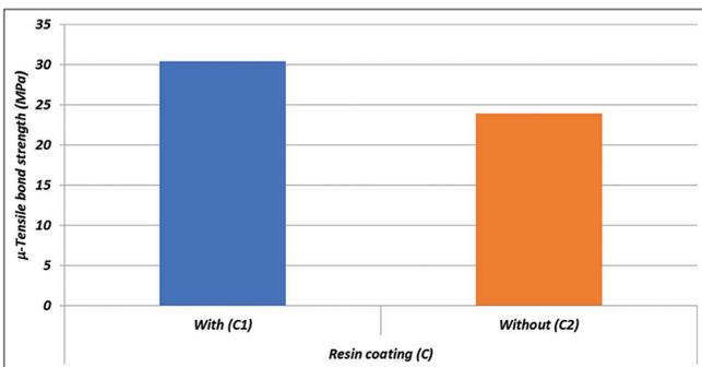
Figure 8: Column chart of total  $\mu$ -tensile bond strength mean values as function of resin coat application
