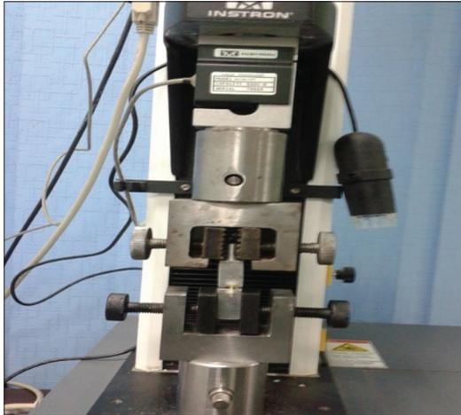
Figure 7: Universal testing machine
