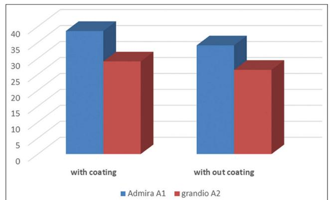
Figure 9: Column chart of  $\mu$ TBS mean values for all composite groups as function of resin coating with Etch and rinse application mode
