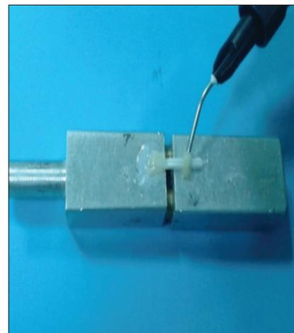
Figure 6: Resin-dentin beam holder
