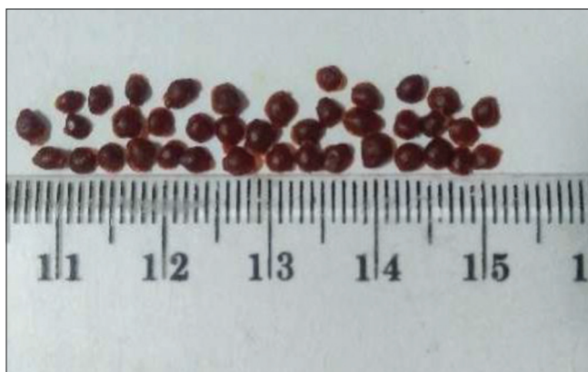
Figure 1: Photo of alginate beads containing turmeric extract solid dispersion (turmeric extract- polyvinylpyrrolidone). The diameter of beads was about 1.5 mm
