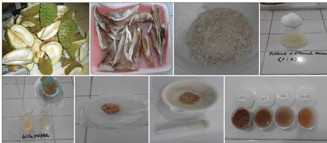
Figure 1: The process extraction of durian peel
