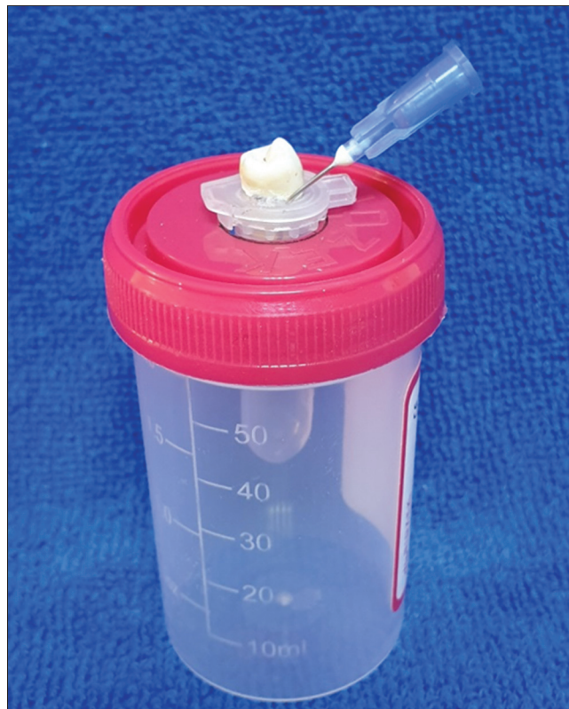
Figure 1: Photo illustration of the collecting apparatus: Tooth, collecting Eppendorf tube, plastic container, and ventilating needle
