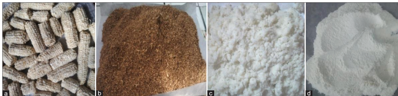
Figure 1: CCM manufacturing process; (a) corncob, (b) corncob powder, (c) corncob alpha-cellulose, and (d) CCM. CCM: Corncob cellulose microcrystal
