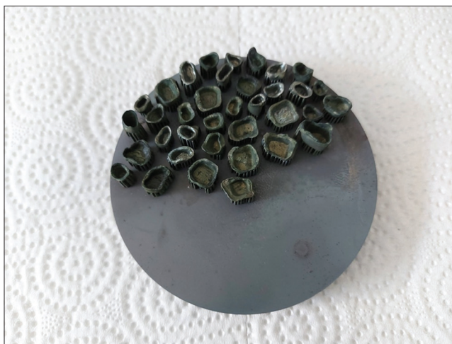
Figure 1: Metal copings after DMLS
