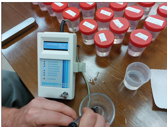
Figure 2: Apparatus Dentotest Six for E_{ocp} evaluation
