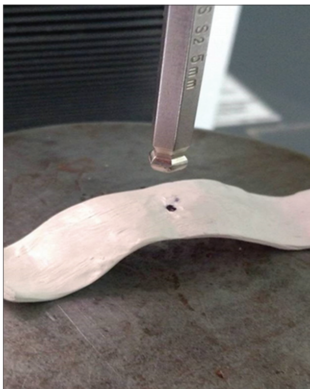
Figure 4: BioHPP® palatal strap showed complete extension deformation after performing fracture resistance test
