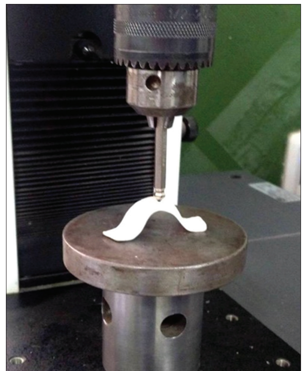
Figure 3: BioHPP® palatal strap during fracture resistance test using universal testing machine
