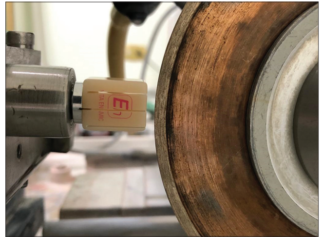
Figure 1: Enamic block cutting
