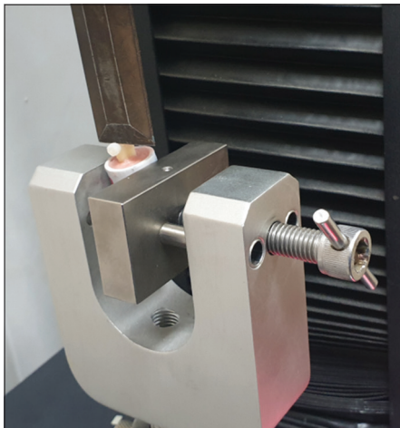
Figure 1: Photo of the Instron testing machine used to measure the shear bond strength of the prepared samples
