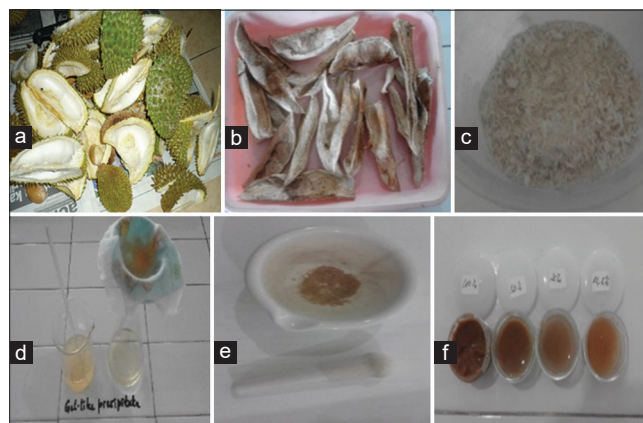
Figure 1: The process of PG synthesis of durian peel extract from (a) raw material (a), (b) dried, (c) blended, (d) precipitated, (e) powdered, and (f) PG durian extract
