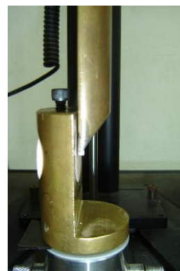
Figure 3: Specimen during shear bond strength testing
