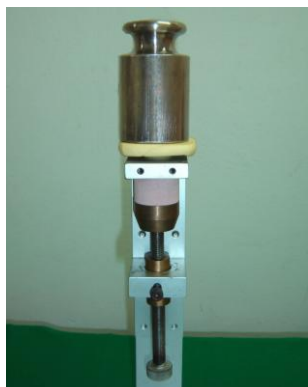
Figure 2: Load application during bonding
