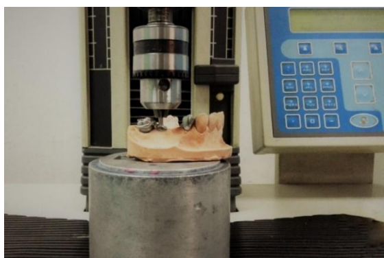
Figure 3: The testing machine with one of the specimens
