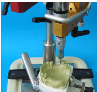
Figure 1: Formation of guiding surfaces
