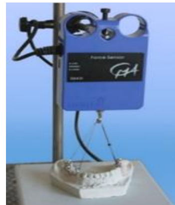
Figure 3: Measurement of retention force
