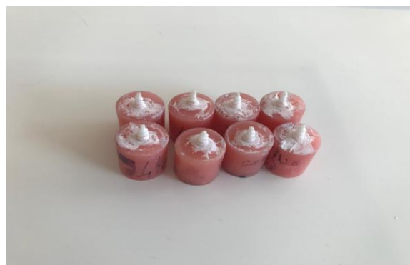
Figure 2: Zirconium post systems, cemented in acrylic blocks
