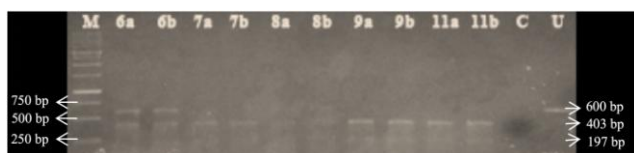
Figure 1: Result of analysis of the cutting region in BspHI restriction enzyme of Met420del polymorphism in SLC22A1 gene; aa homozygous/mutant (lane 7a-11b: 403bp and 197bp), Aa heterozygous variants (lane 6a and 6b: 600bp, 403bp, and 197bp). Note: lane M = marker/ladder 1 kbp; lane 6a and 6b = samples of heterozygote type in; lane 7a-11b = samples of mutant type; lane C = negative control; lane U = undigested sample
