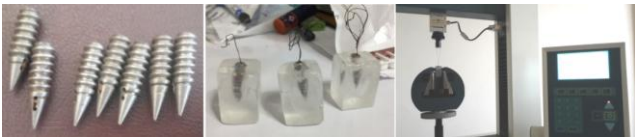
Figure 6: Test samples and one sample during testing on Universal Testing machine
