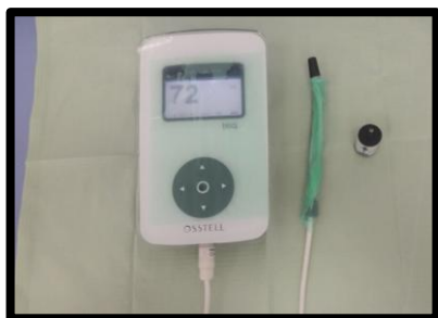
Figure 1: Showing Osstell™ device used in Resonance frequency analysis of implants
