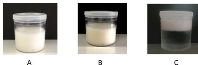
Figure 2: Appearance of the prepared sunscreen emulsion containing sunflower oil; A) Before storage; B) After storage for 8 weeks; and C) After storage for 12 weeks) at room temperature
