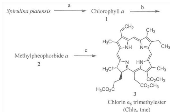
Figure 2: Chlorophyll a extraction from *S. platensis* and its transformation into Ce6 trimethylester; A) Dry spirulina mass, acetone, N<sub>2</sub> (liquid), ca, 60 min, then warm up to room temperature, acetone, reflux, 24 hours; B). H<sub>2</sub>SO<sub>4</sub> conc, MeOH, Ar, rt, 20 hours. (c). 1M KOH in MeOH, THF/CHCl<sub>3</sub>, Ar, rt, 30 min (73%) or KOMe, MeOH, acetone, Ar, rt, 30 min, 85%
