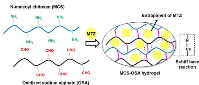
Figure 1: Schematic of in situ drug loading in MCS-OSA hydrogels via Schiff base cross-linking reaction
