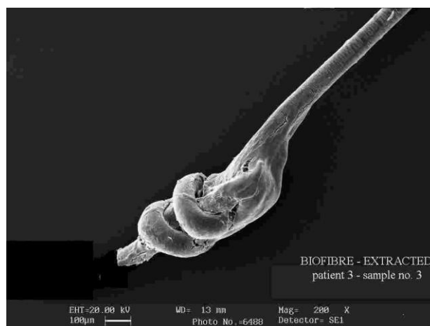
Figure 6: a Reversible knot of Biofibre® after extraction. No remains stay embedded on the scalp, allowing prompt restitution ad integrum of scalp
