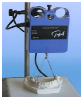
Figure 3: Measurement of retention force
