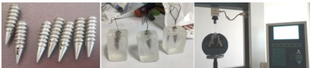
Figure 6: Test samples and one sample during testing on Universal Testing machine
