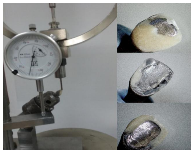
Figure 1: Testing the samples with universal test machine (Tritech of 10056) and their fracture localisation
